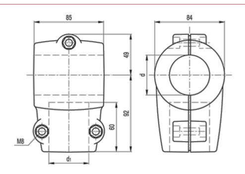
d (inch) = 2 Gas d1 (inch) = 1 1/4 Gas d1 (mm) = 42.4 d mm = 60.3 Weight (g) = 380
